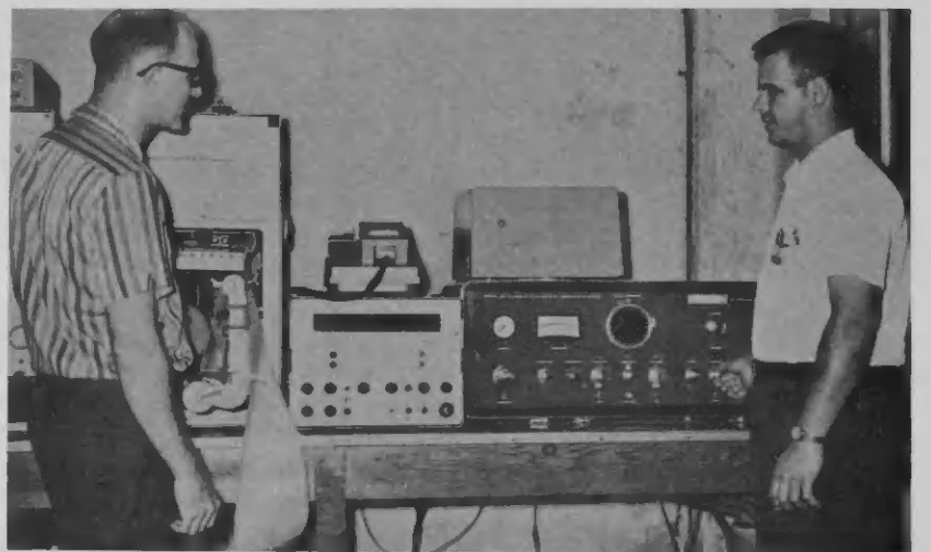
PETE SCHERMERHORN and Felix Croes (r) check operation of new temperature programmed gas chromatograph, coupled to electronic integrator and printing machine.
